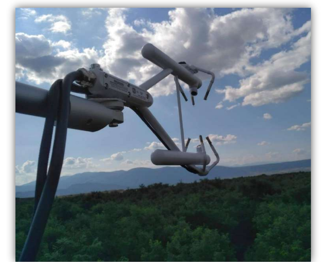
Figure 2: The CO 2 /H 2 O analyser at the top of the tower
